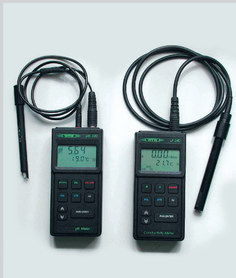
Dampening system monitoring tools include digital conductivity meter, pH meter and probe thermometer (digital devices are more accurate and easier to calibrate). Photo Sun Chemical.
