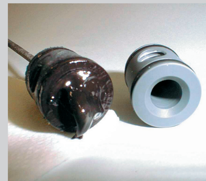
An inline ejector nozzle contaminated with ink from either using the wrong filter element or poor maintenance. Photo Technotrans.
