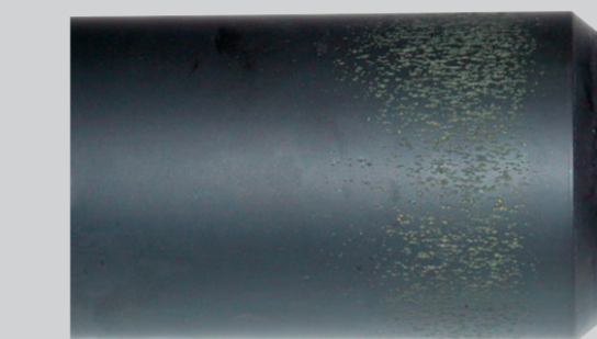
Roller damaged due to uneven setting that has significantly increased running temperature. Photo Böttcher.
