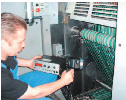
A strobe scope is a useful tool to help identify running problems on moving equipment. Photo manroland.
