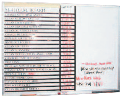
An autonomous maintenance board is kept up to date by the press crew to help prioritise their maintenance actions. These are made either at planned maintenance periods with smaller tasks during press stops. Photo Quad Graphics.
